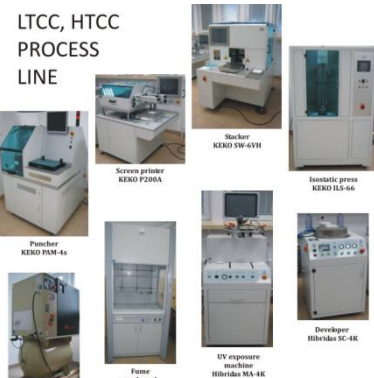
Fig. 2. Technological line for LTCC and HTCC
